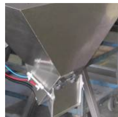
Discharge chute + timing hopper
