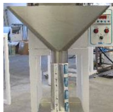
Additional discharge chute
