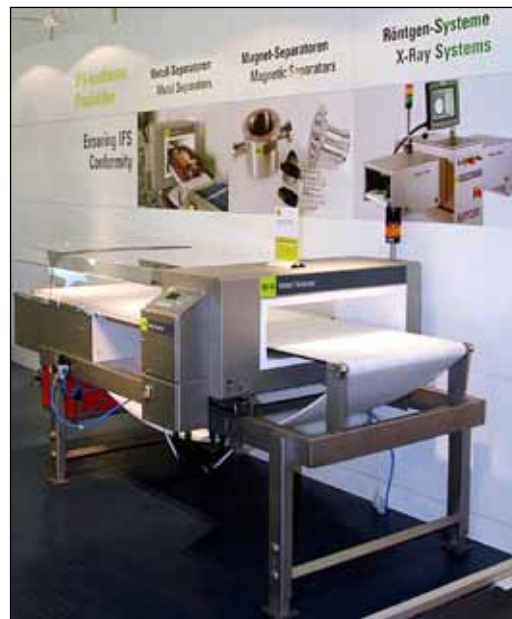
UNICON metal detection system with retracting belt
