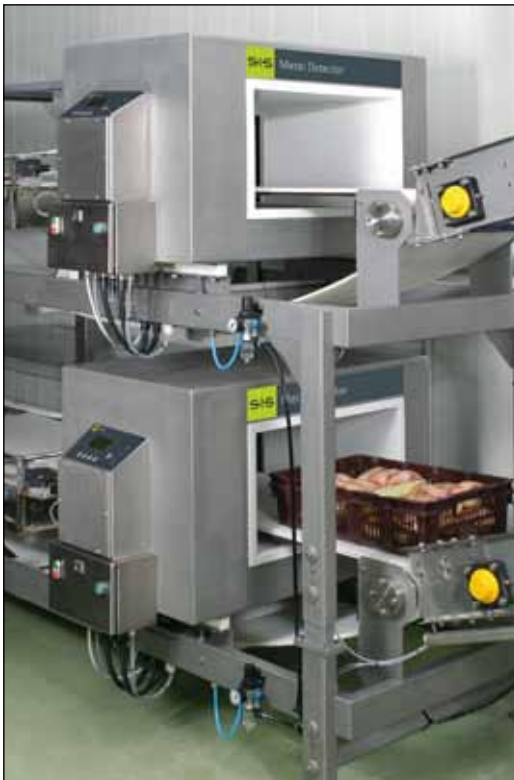
Metal inspection of poultry in E1 containers
