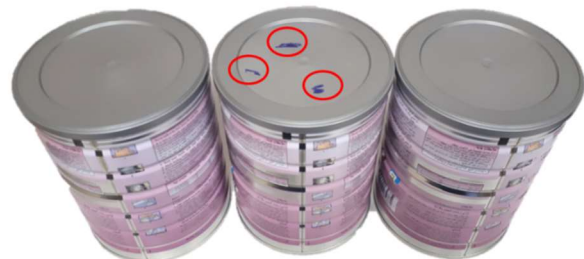
DEFECTIVE CAPS, SCRATCHED OR DIRTY - REJECTED
