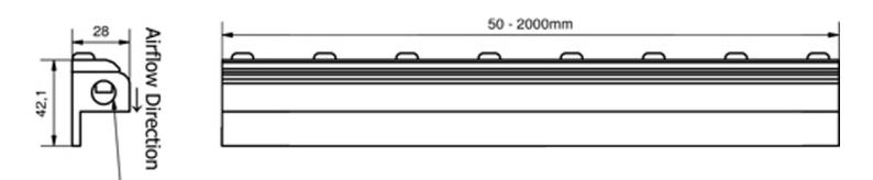
1/4"bsp female air entry at each end. units over 600mm have intermediate ports along rear of air curtain.
