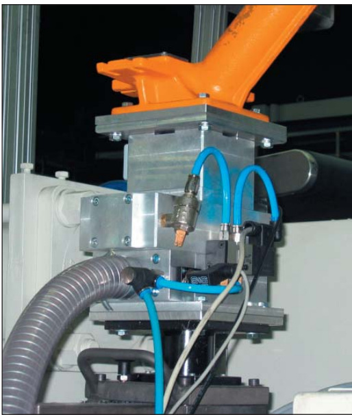
PROTECTOR metal separator installed at the material inlet of an injection-moulding machine
