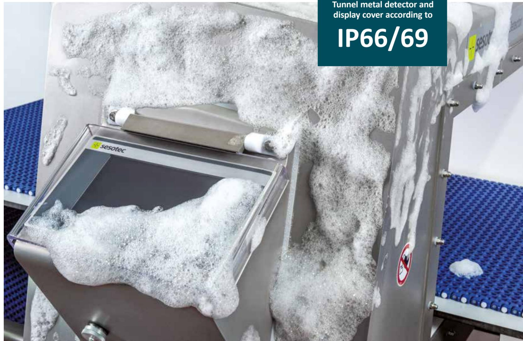
Tunnel metal detector and display cover according to **IP66/69**
